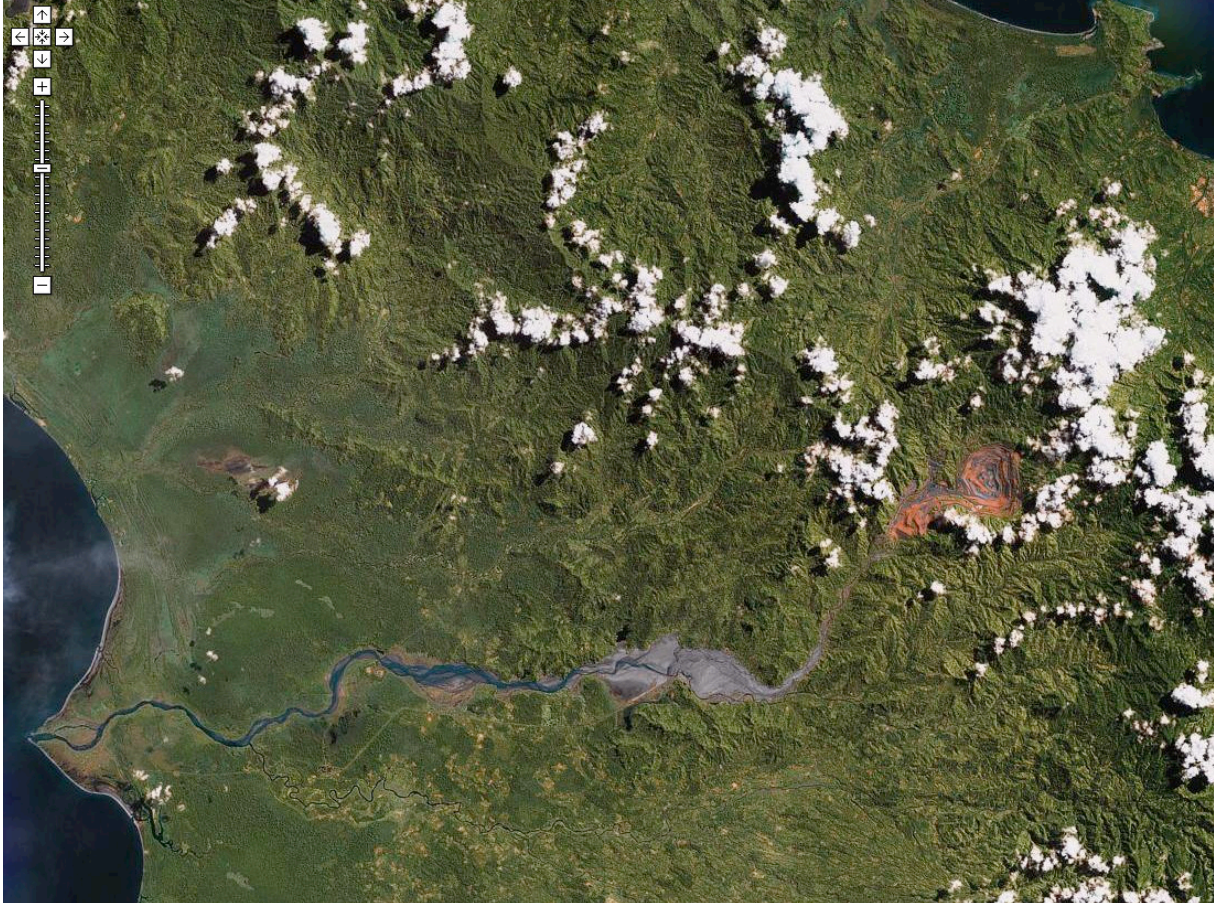
The Panguna mine's tailings area around the Jaba river seen from a satellite (brown = mine, grey = tailings)
